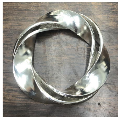
Fig. 29. The antenna variant, manufactured by means of casting method.
