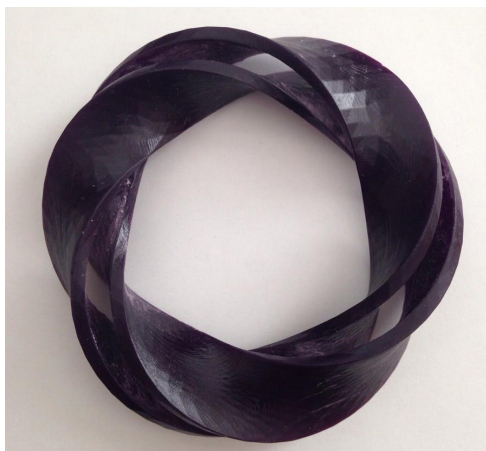
Fig. 28. Antenna made of the conductive plastic using 3D printing method
